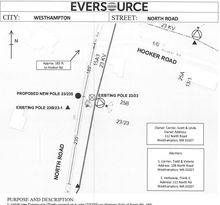
1. Install new Eversource (Solely owned) stub pole (23/23S) on Western Side of North Rd. 185' south of the centerline on Hooker Rd. and 35' opposite side of North Rd from existing pole 23/23.
